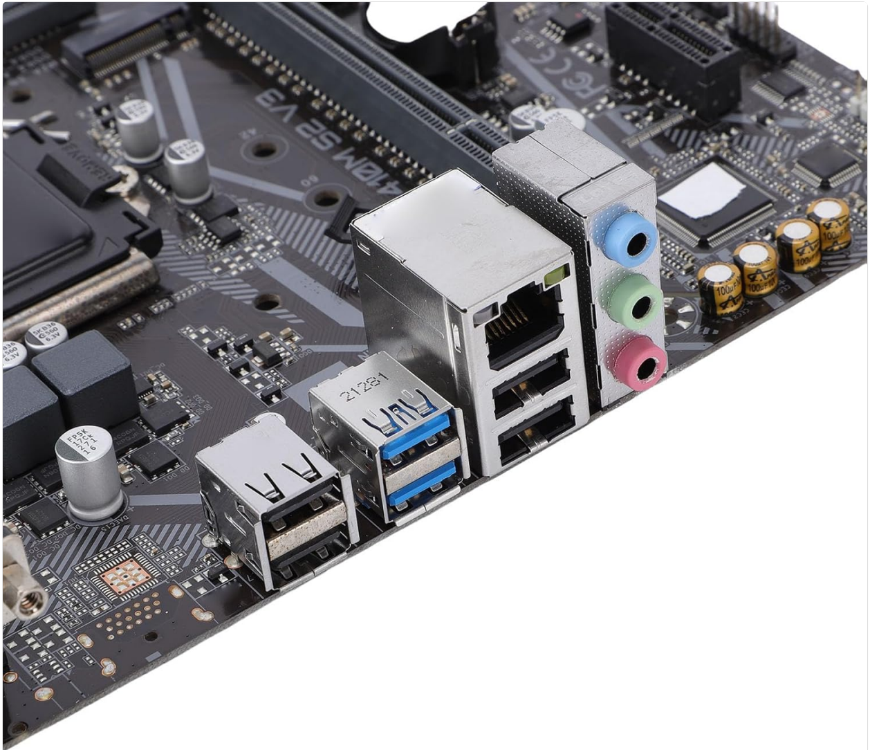
Figure 3.3: Rear I/O panel with USB, Ethernet, and audio ports.
