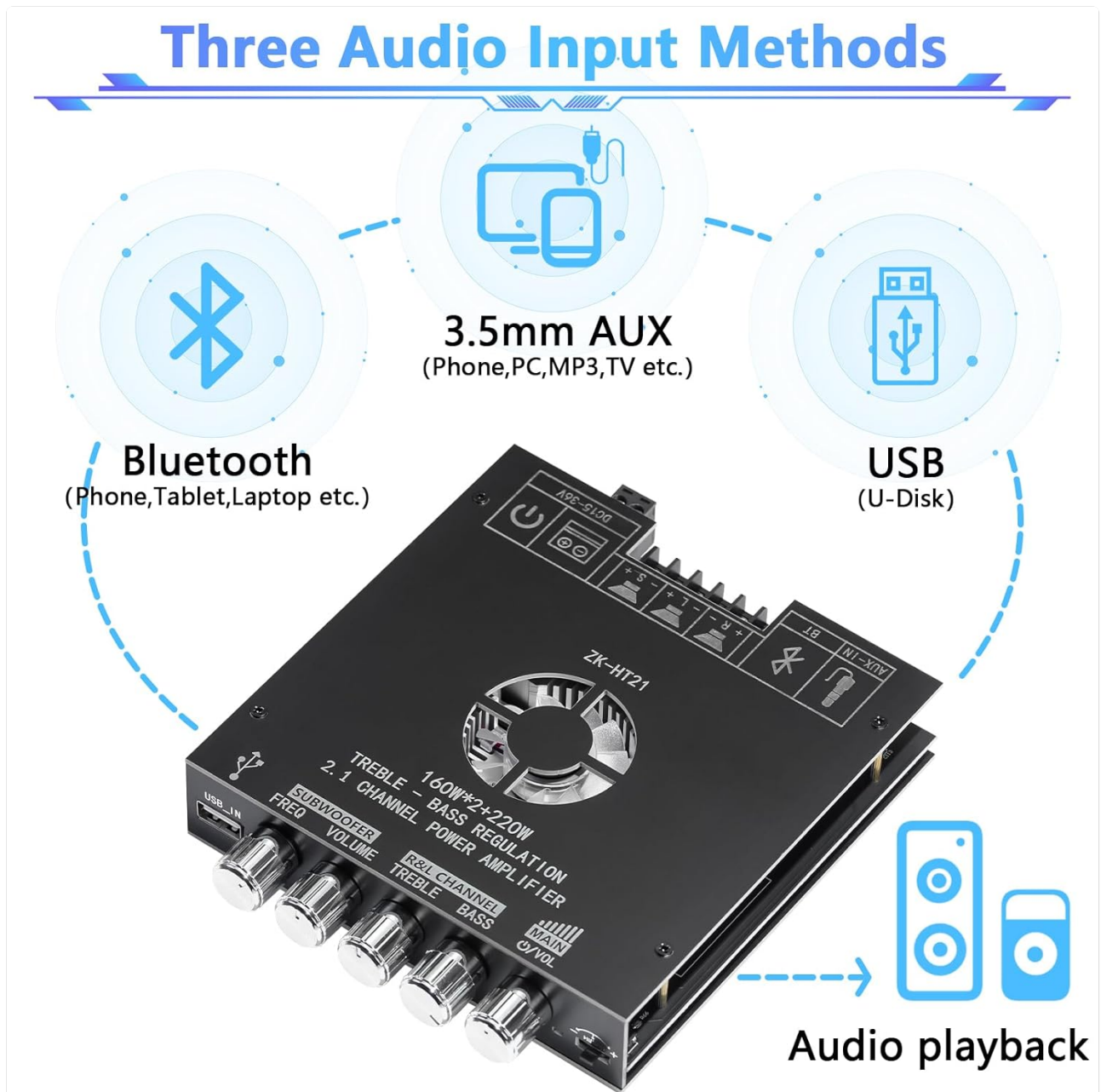
Figure 6.1: Audio Input Methods. This image visually represents connecting audio sources via Bluetooth, AUX, or USB to the amplifier board for playback through speakers.
