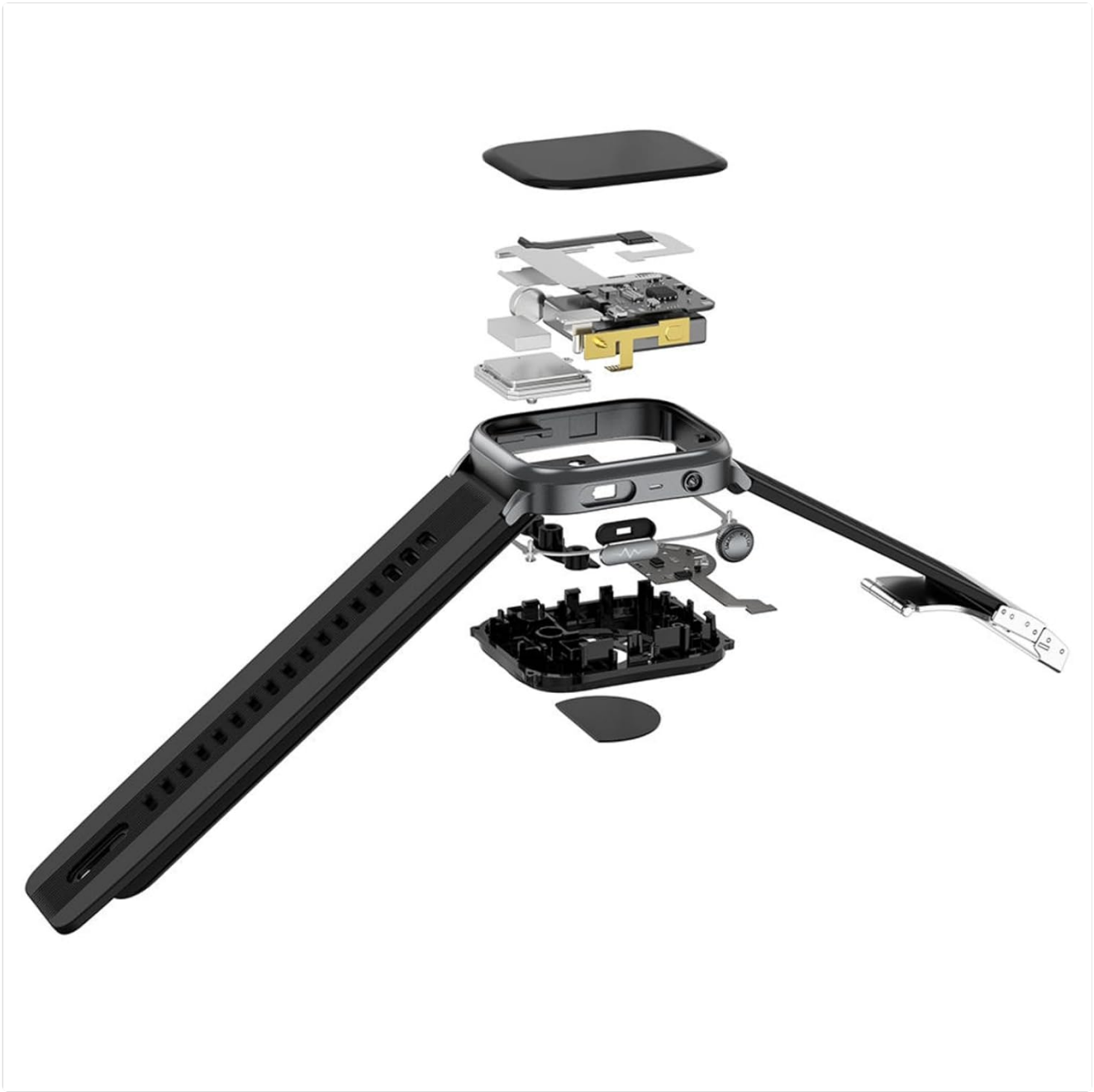
Image: An exploded view illustrating the internal components of the TK66 Smart Watch.
