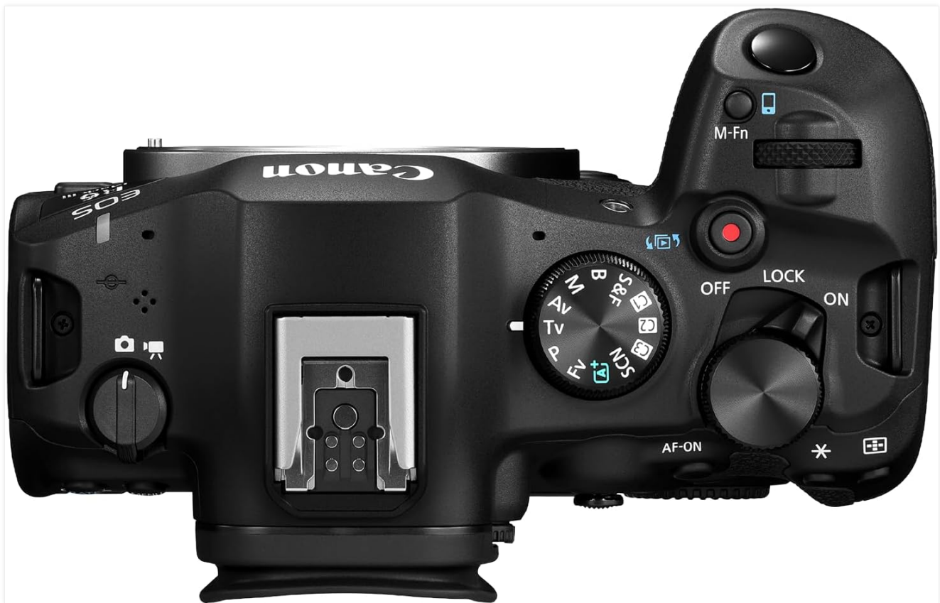
Figure 4.1: Top view of the Canon EOS R6 Mark III, highlighting the mode dial and power switch.
