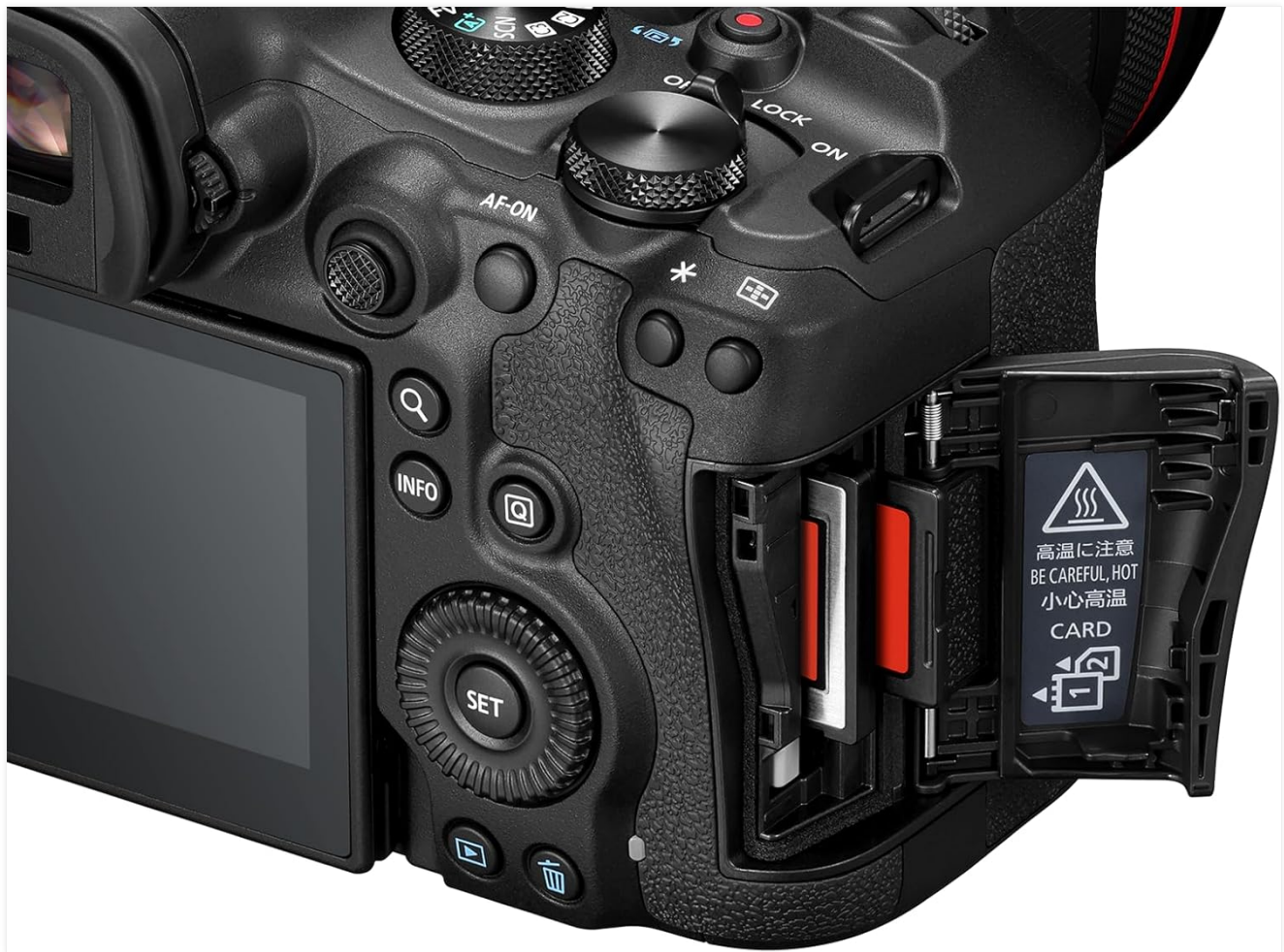
Figure 3.2: The dual memory card slots of the EOS R6 Mark III, supporting CFexpress Type B and UHS-II SD cards.
