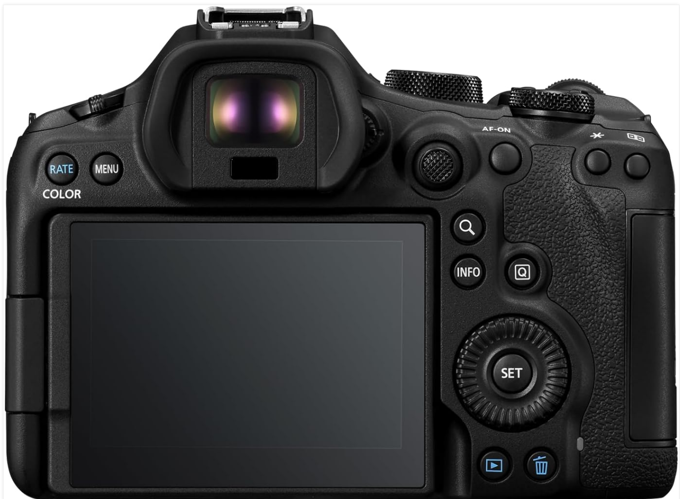
Figure 4.2: Rear view of the Canon EOS R6 Mark III, showing the articulating LCD screen and control buttons.
