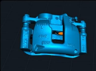
Figure 3: Volumetric accuracy of 0.02\text{mm} + 0.08\text{mm/m} demonstrated on complex mechanical parts.
