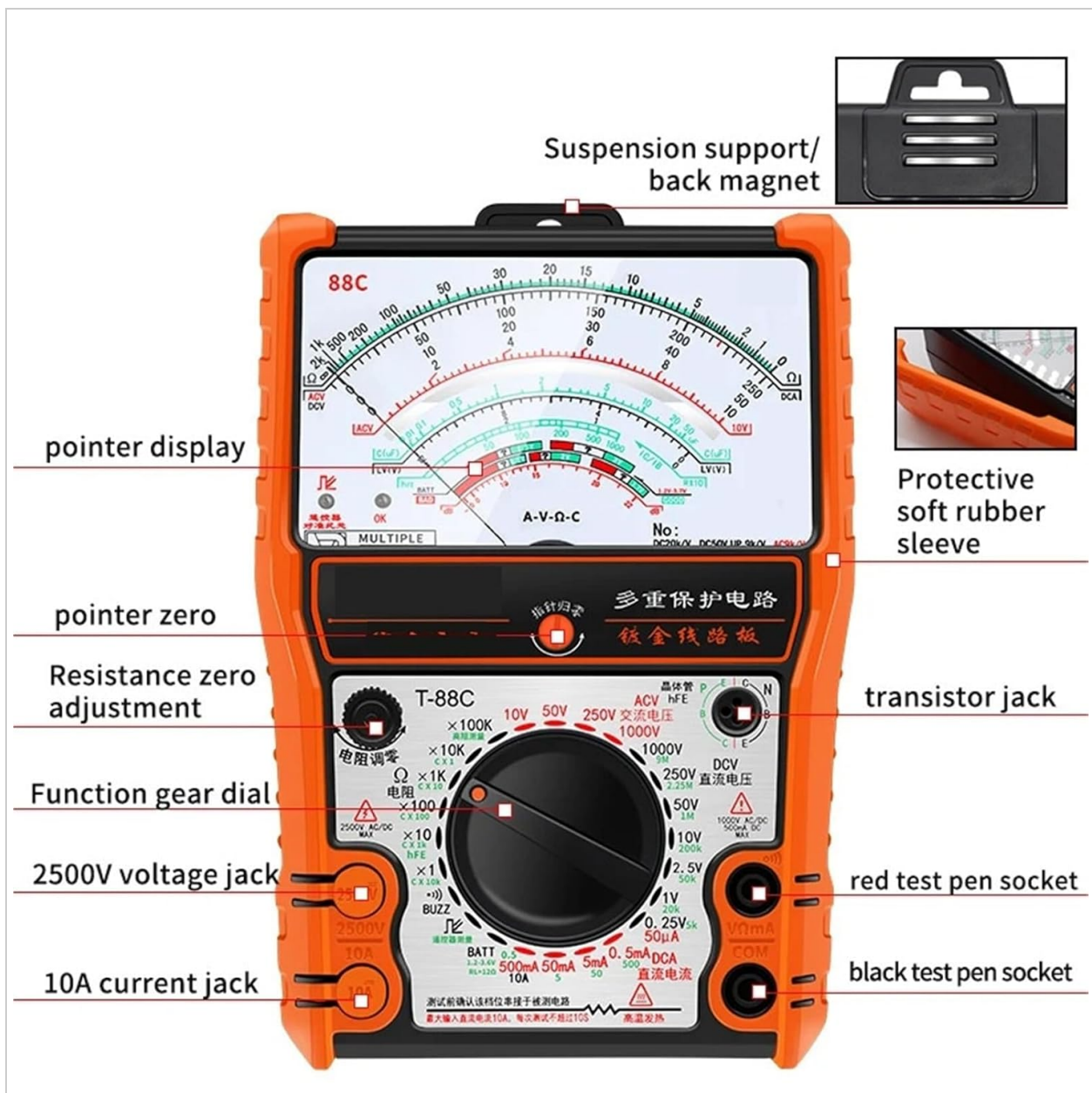
Figure 3.2: Labeled components of the T88C Multimeter.
