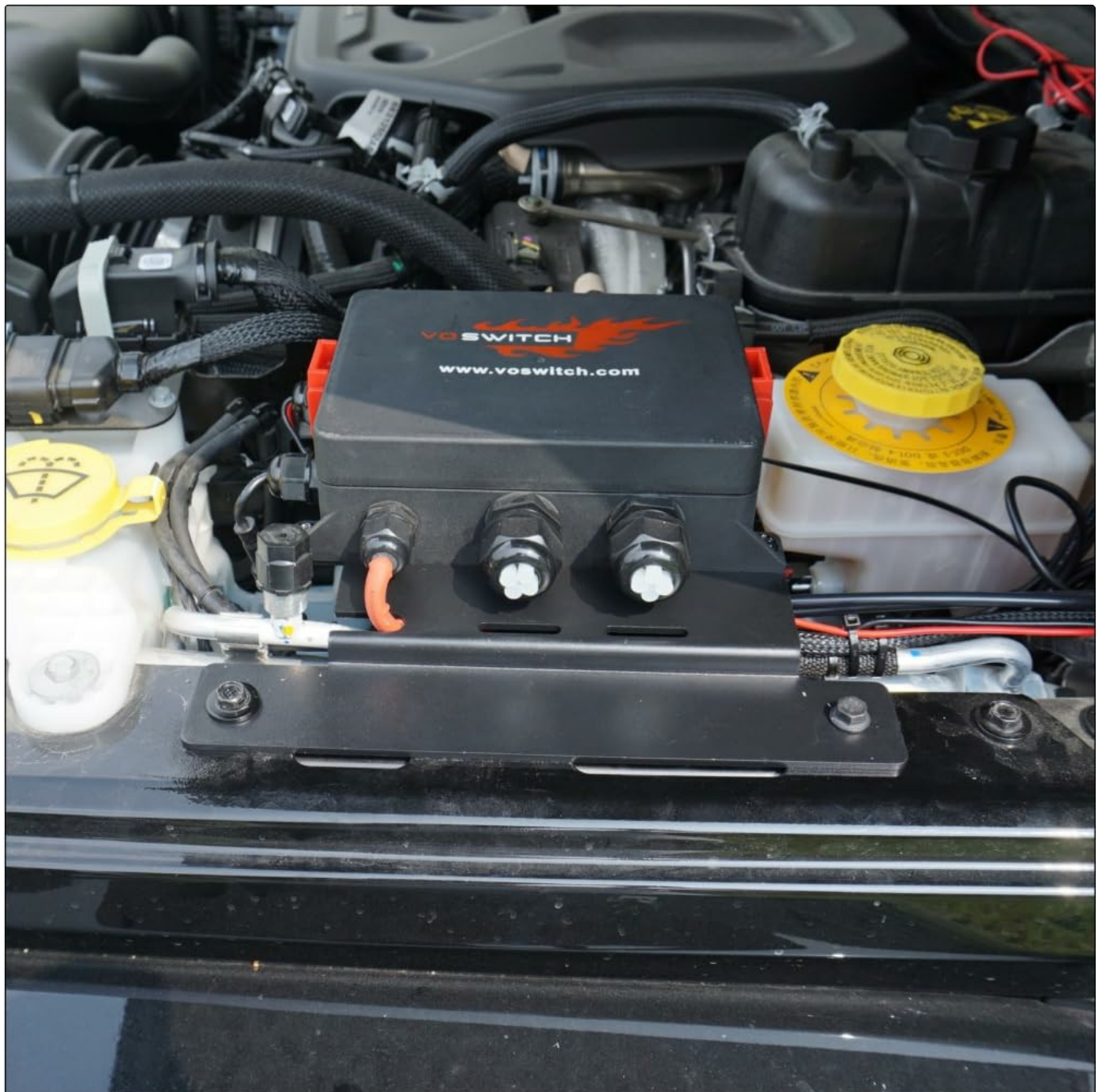
Image 4.2: Wiring Connections. This image provides a closer look at the power module and its wiring connections, illustrating the pre-wired harness design.
