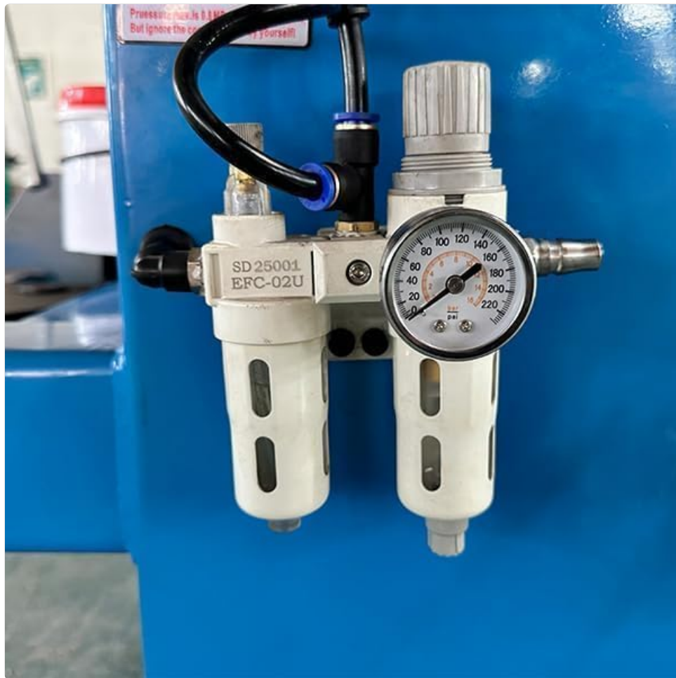
Image: A close-up of the air pressure gauge and filter system on the KATOOL Tire Changer, indicating the machine's pneumatic controls.
