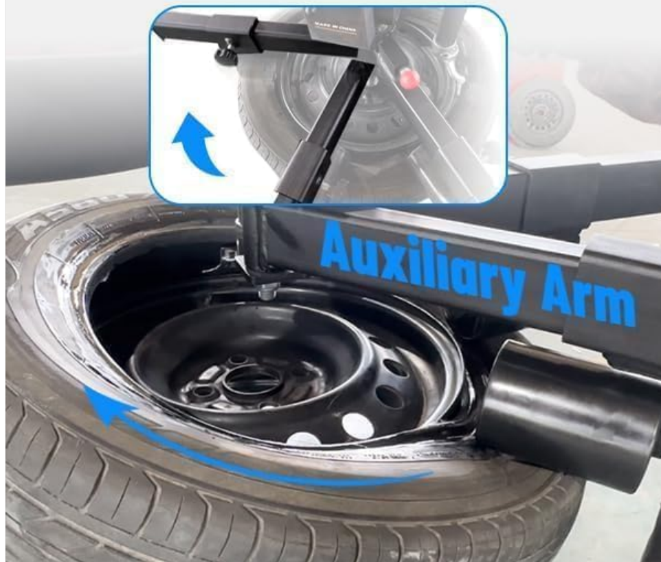
Image: The auxiliary arm of the KATOOL Tire Changer is shown in action, assisting in the removal of a tire from the rim, demonstrating how it helps lift and manipulate the tire bead.
