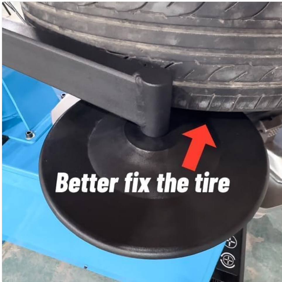
Image: The KATOOL Tire Changer's bead press tool is shown fixing the tire bead onto the rim, ensuring a secure fit during the mounting process.
