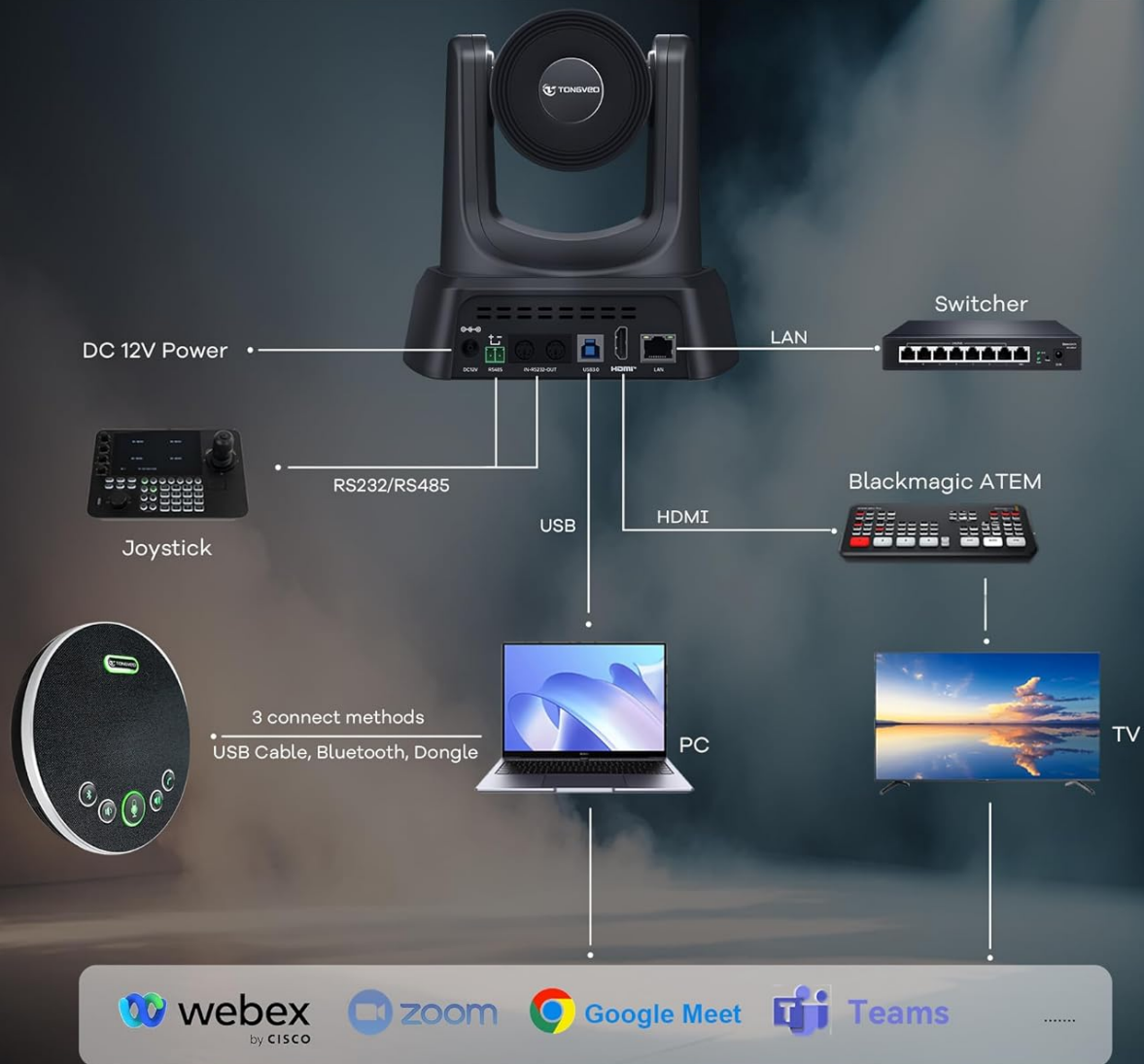
Image: Rear ports of the TONGVEO PTZ camera, illustrating diverse connectivity options.
