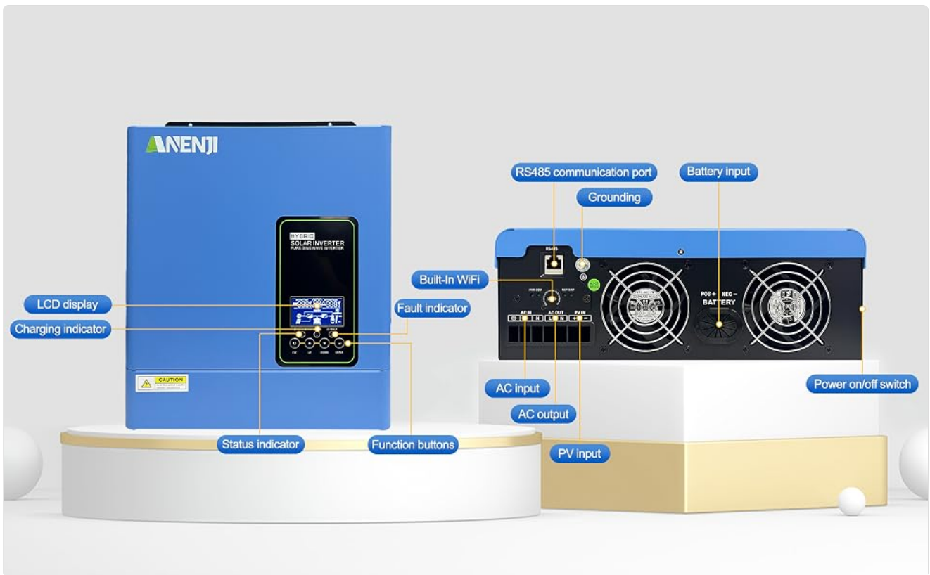
Figure 6: Detailed Component Diagram of the Inverter.
