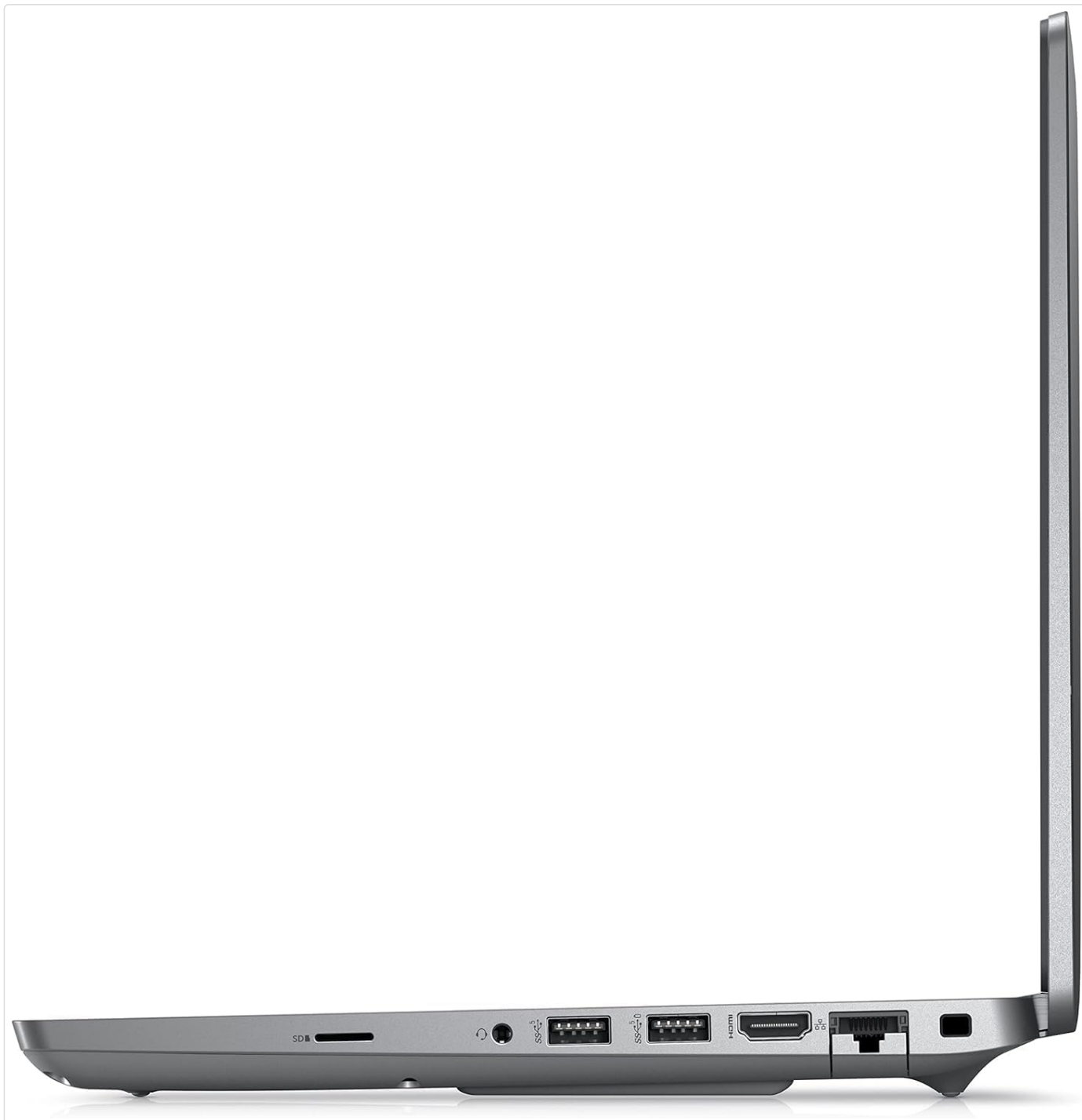
Figure 3: Right side ports including USB, HDMI, and Ethernet.
