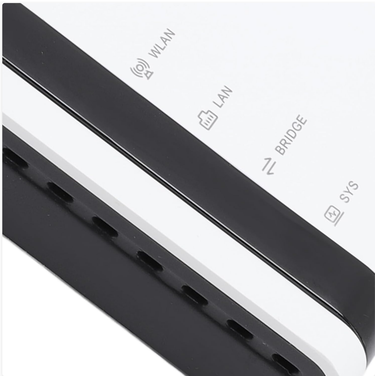
Image 5.1: The top panel of the print server features indicator lights for WLAN (Wireless LAN), LAN (Wired LAN), BRIDGE, and SYS (System status), providing visual feedback on the device's operational status.
