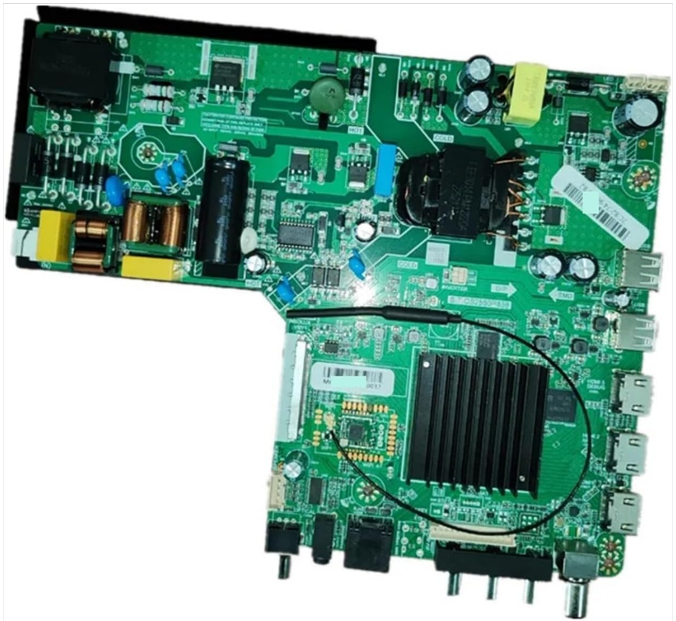
Figure 3.3: Angled view of the S.T.CS2560P838 TV Motherboard. This perspective provides a clearer view of the heatsink covering the main processor, indicating thermal management. Various ports, including multiple HDMI inputs, USB ports, and coaxial antenna inputs, are clearly visible along the edges of the board, demonstrating its connectivity options.
