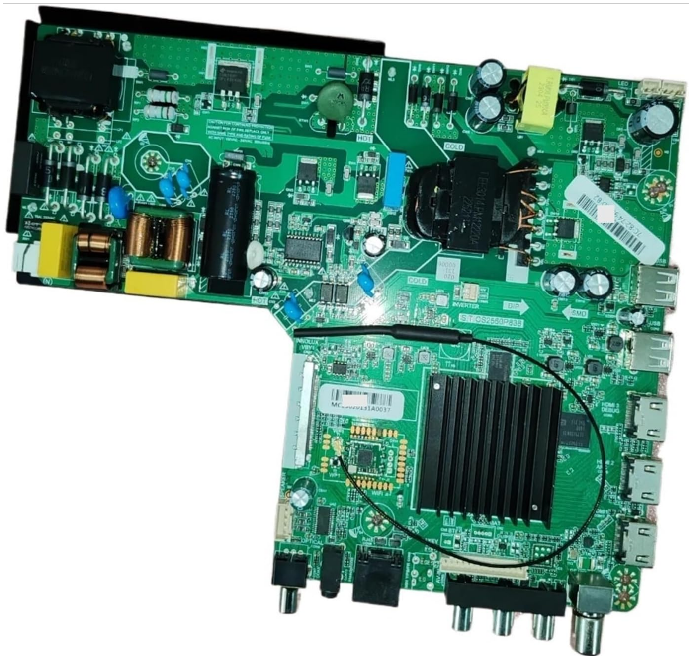
Figure 3.4: Detailed angled view of the S.T.CS2560P838 TV Motherboard. This image offers a closer look at the intricate circuit design and component placement. Key features like the WiFi antenna connection (black wire), various capacitors, inductors, and integrated circuits are visible, emphasizing the board's complex engineering and compact design.
