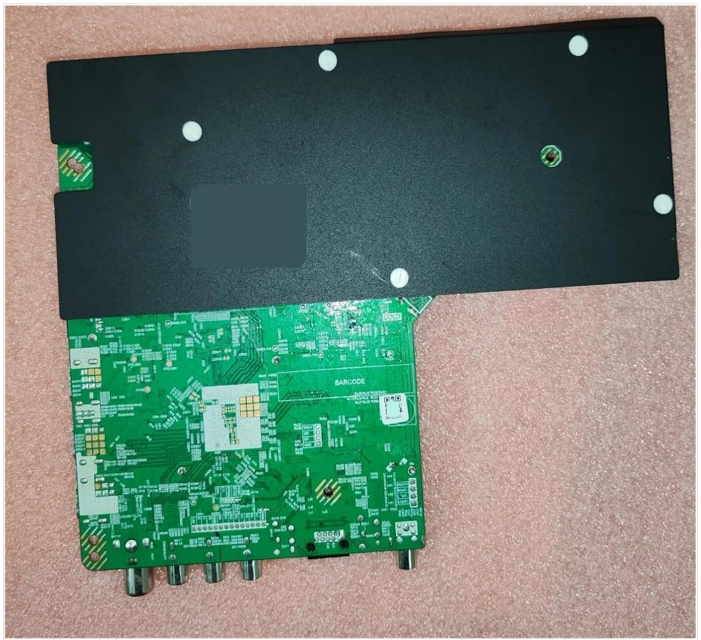
Figure 3.2: Bottom view of the S.T.CS2560P838 TV Motherboard. This image shows the underside of the motherboard, partially covered by a black protective shield. Visible areas include solder points, additional circuit traces, and mounting holes. The protective cover helps to shield sensitive components and provides structural integrity.
