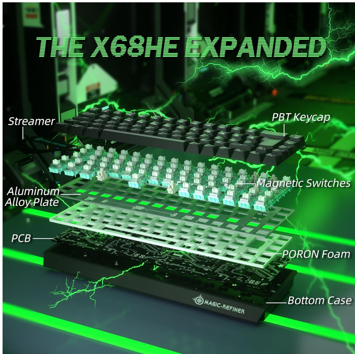
Figure 2.4: Exploded diagram illustrating the internal components of the X68 HE, including PBT keycaps, streamer, aluminum alloy plate, magnetic switches, PCB, and PORON foam.
