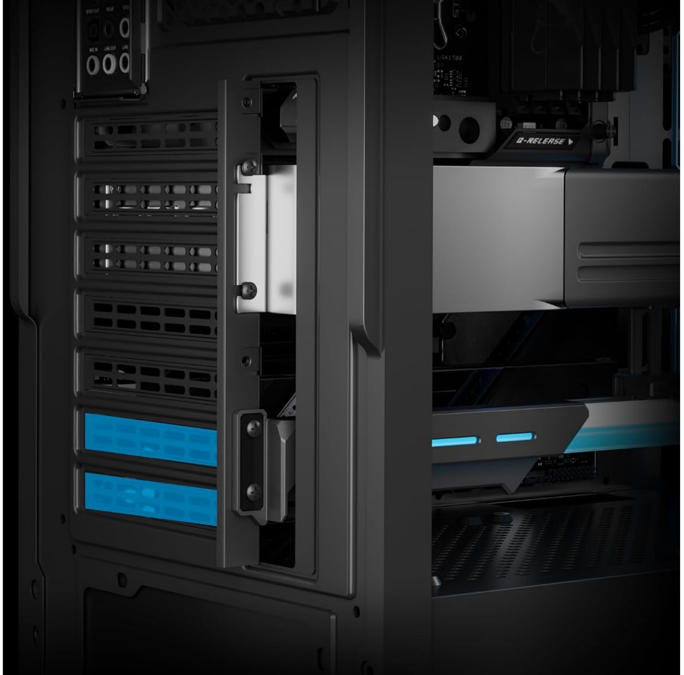
Image: The GPU brace installed, demonstrating its minimal PCI slot usage.
