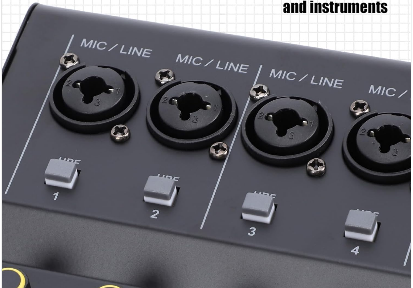
Image: Detail of the multi-channel audio input interfaces, showing XLR/6.35mm combo jacks for microphones and instruments.
