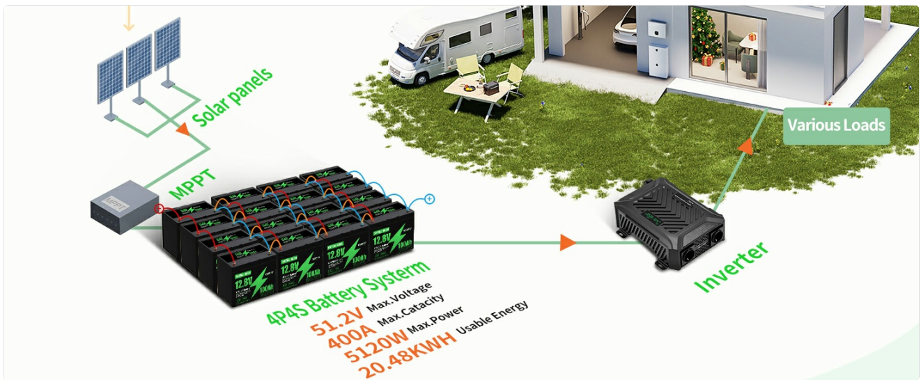
Image 4.1: Diagram illustrating how to connect multiple batteries in series and parallel for flexible capacity expansion in a solar power system.
