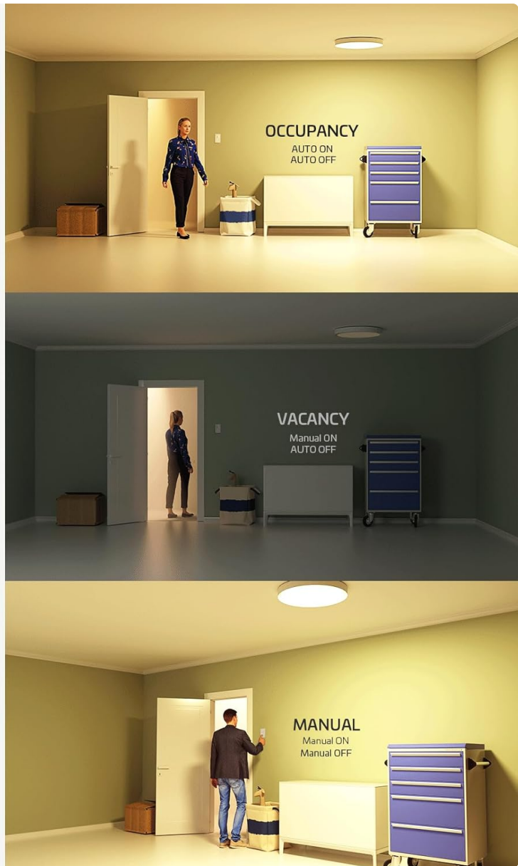
Figure 3: Overview of 3-in-1 Operation Modes
