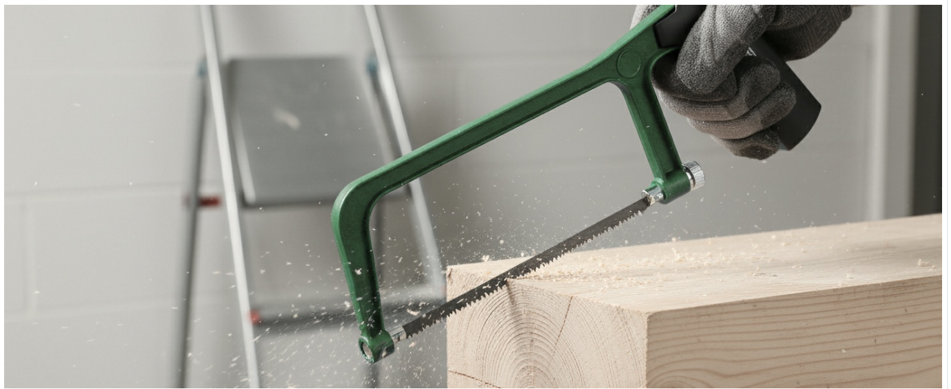
The hack saw is designed for cutting various materials. Always secure the workpiece and use a steady, even stroke.
