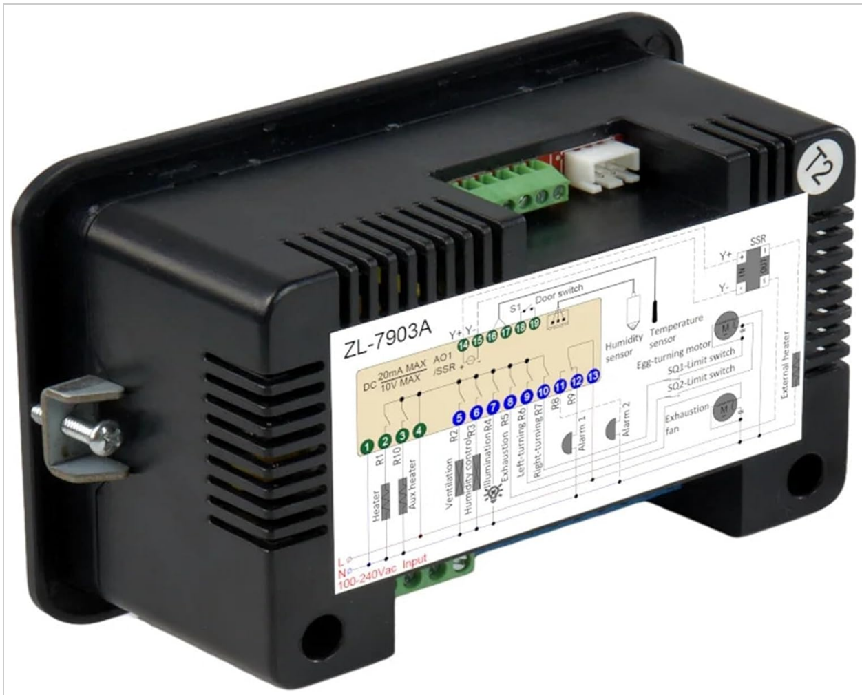
Figure 4.1: Rear view of the ZL-7903A controller, showing the terminal block and an integrated wiring diagram for various connections including power, sensors, and output devices.
