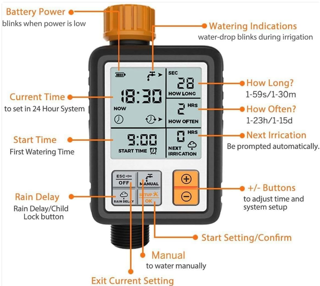
Image 2.1: HCT-311 LCD Display and Control Buttons.
