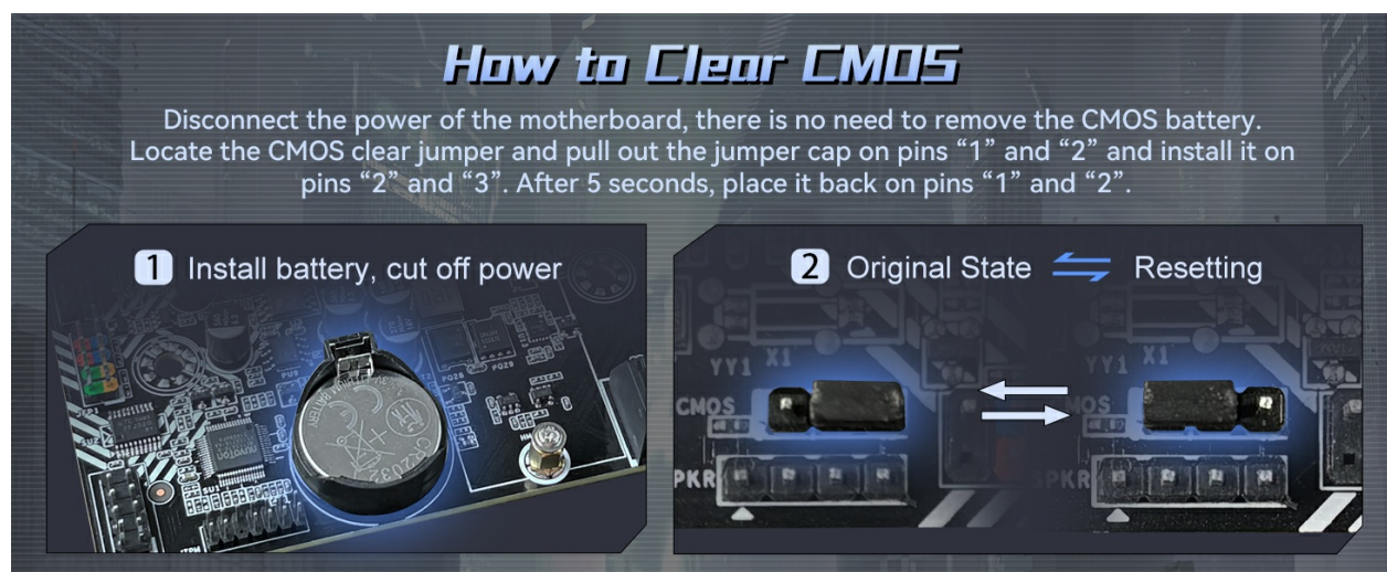
Image: Visual guide on how to clear the CMOS settings on the motherboard.
