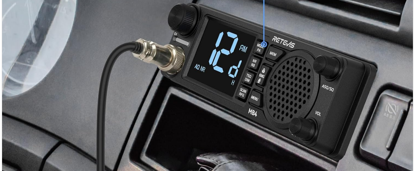
Image: The Retevis MB4 CB Radio mounted in a vehicle's DIN slot.
