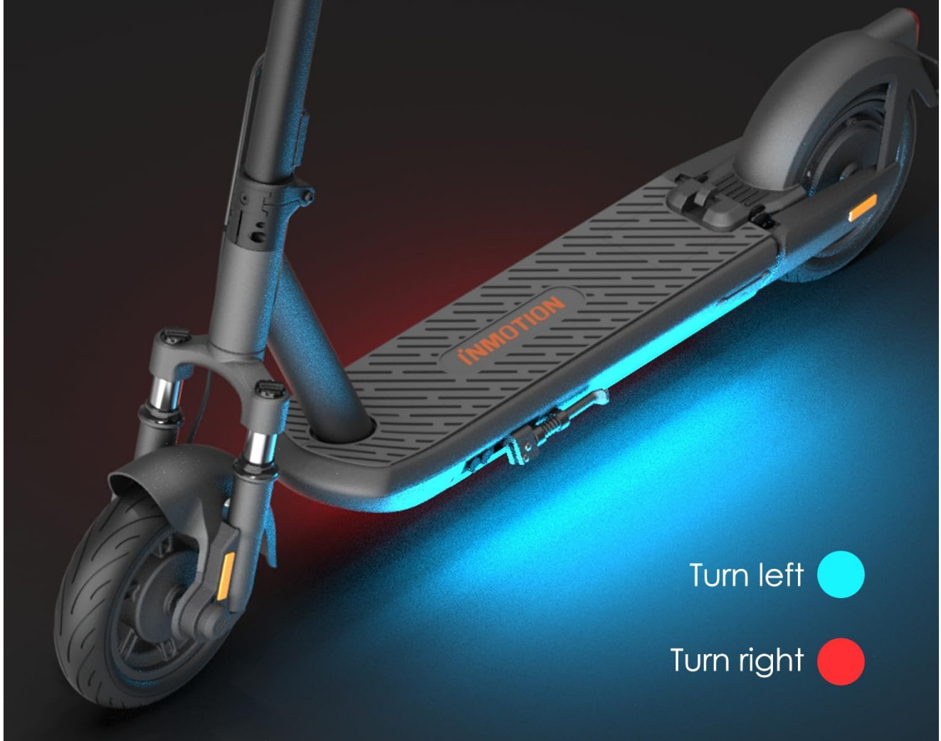
Figure 3.1: The scooter features professional turn signals (blue for left, red for right) for improved visibility and safety.
