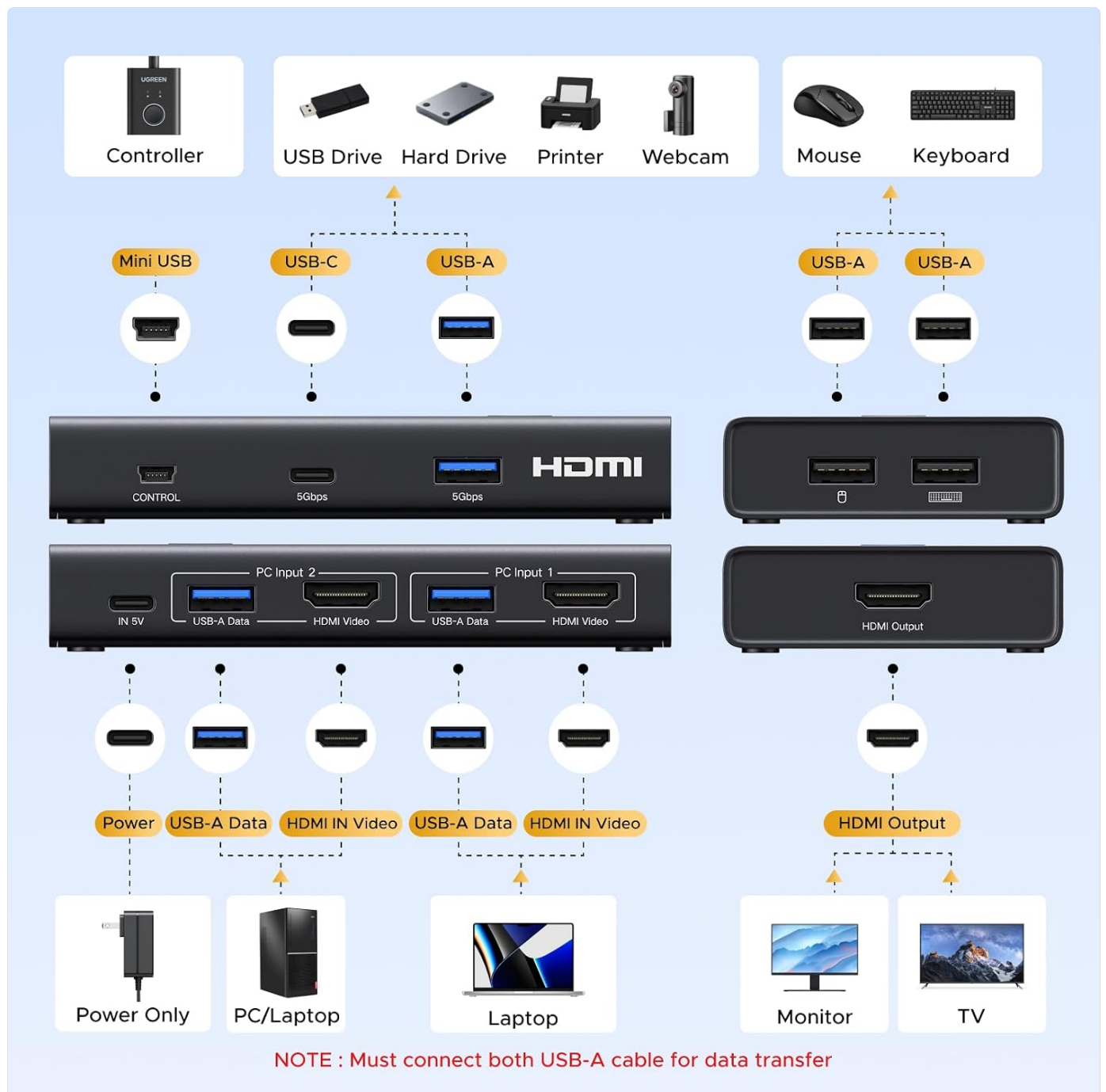
Figure 3.1: Detailed diagram of the UGREEN HDMI KVM Switch showing all input/output ports and their functions. This includes USB-A and USB-C ports for peripherals, HDMI inputs for PCs, HDMI output for the monitor, and a power input.
