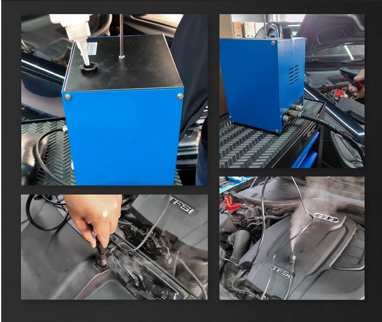
Figure 6.3: Step-by-step visual guide on how to use the Kuntech KT9122 Smoke Leak Detector.
