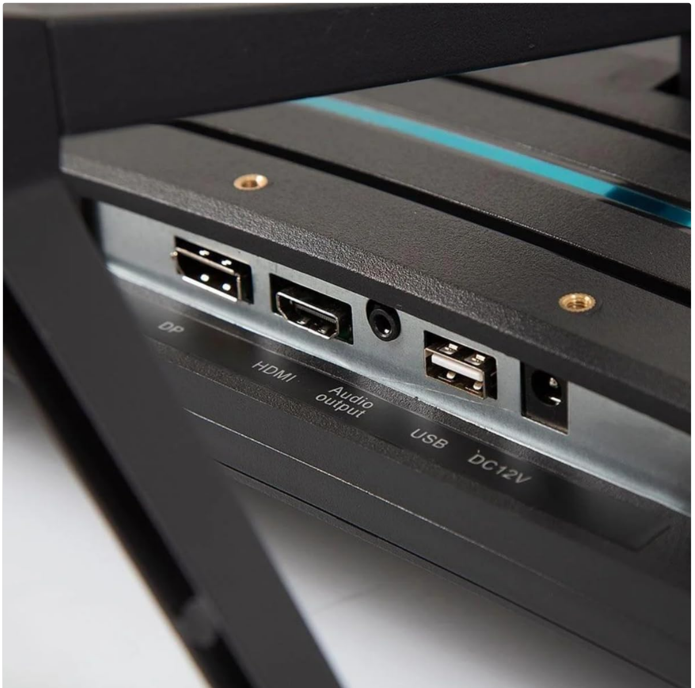
Image: Detailed close-up of the monitor's input/output ports, including DisplayPort (DP), HDMI, Audio Output, USB, and DC 12V power input.
