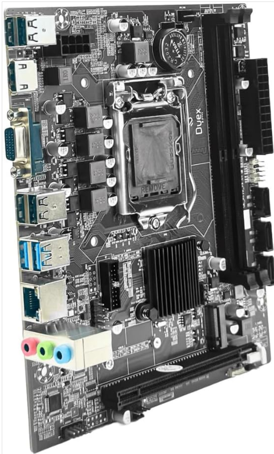
Figure 5.1: Rear I/O panel of the Duex DX-BH110G M2 motherboard, illustrating available ports for peripherals.
