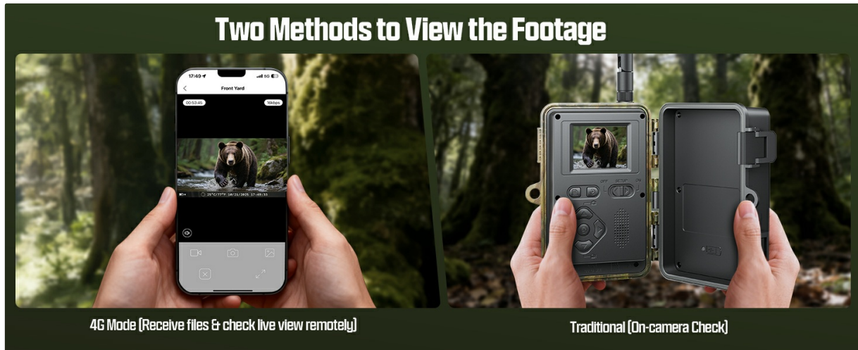
Figure 4: Demonstrating the dual viewing methods: remote via app and direct on-camera.
