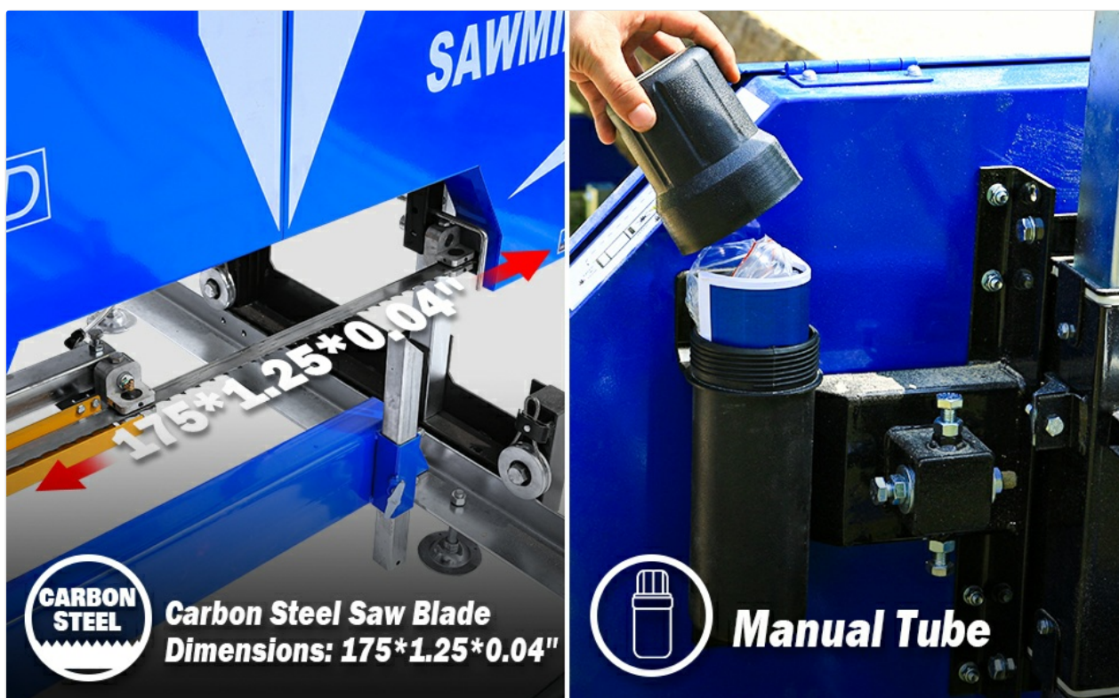
Figure 9: Detail of the carbon steel saw blade and the manual tube for documentation.
