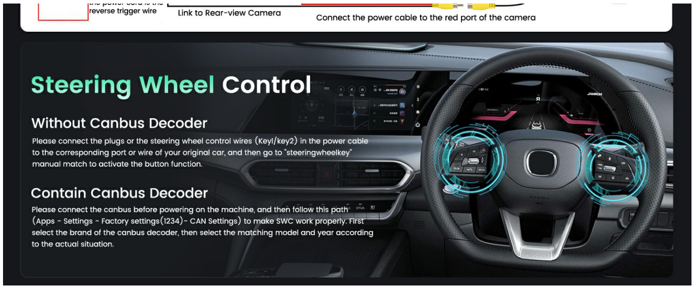
Figure 4.3: Steering Wheel Control Setup. This image explains the setup for steering wheel controls, differentiating between vehicles with and without a Canbus decoder, and providing instructions for connecting the control wires and activating functions.
