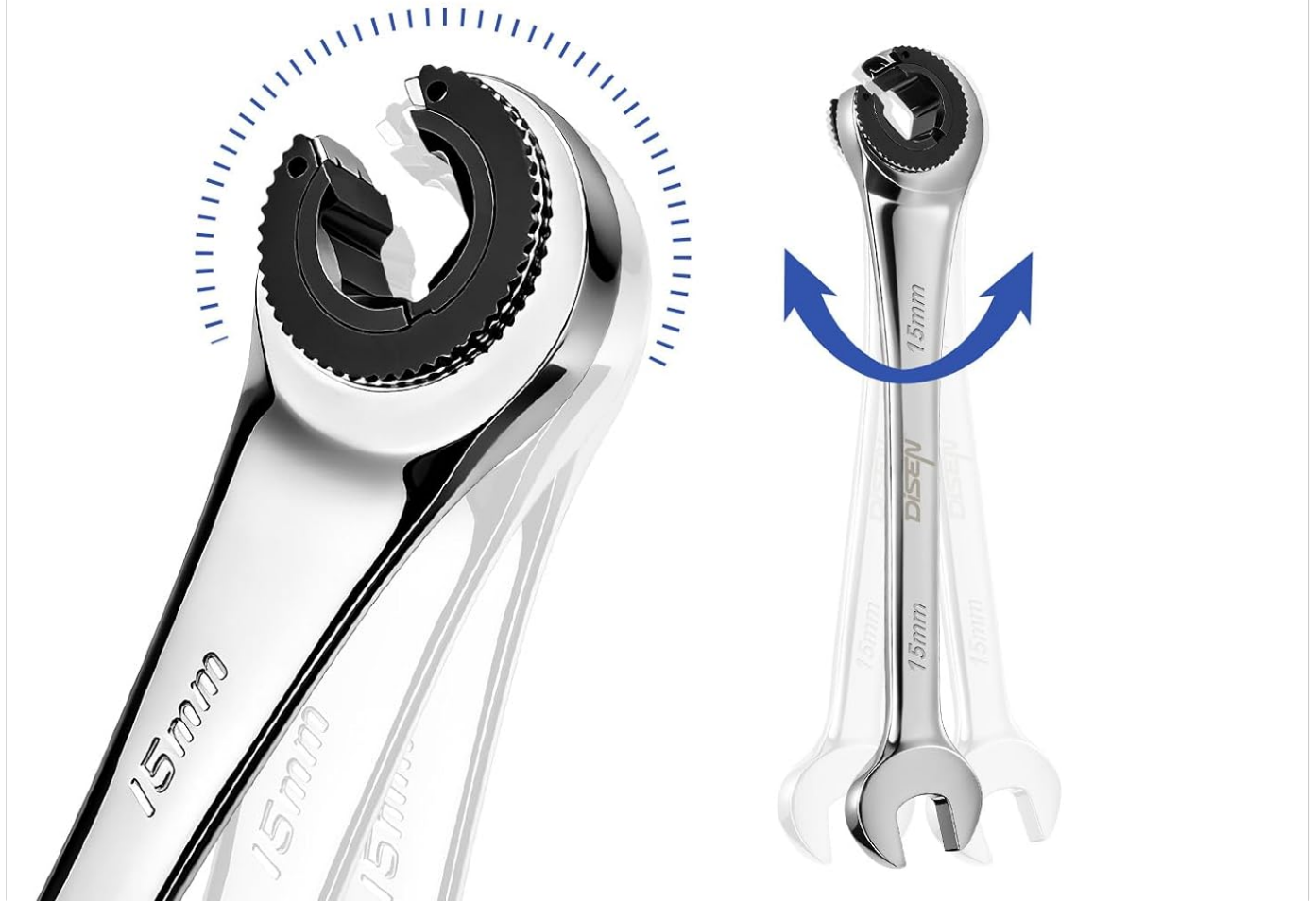
Image 3.2: A detailed view illustrating the 72-tooth ratcheting mechanism and the minimal 5-degree swing arc, which is crucial for working in confined spaces.
