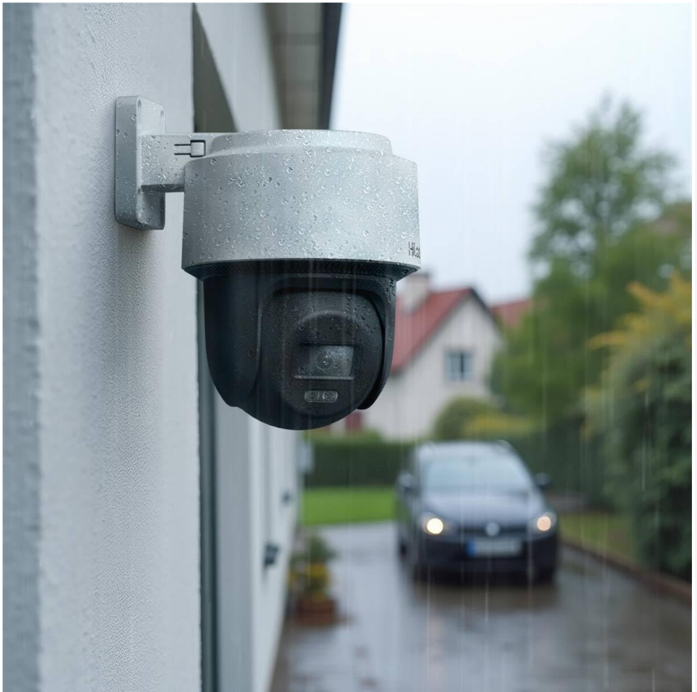
Figure 7: Camera operating in rainy conditions (IP66 rated)
