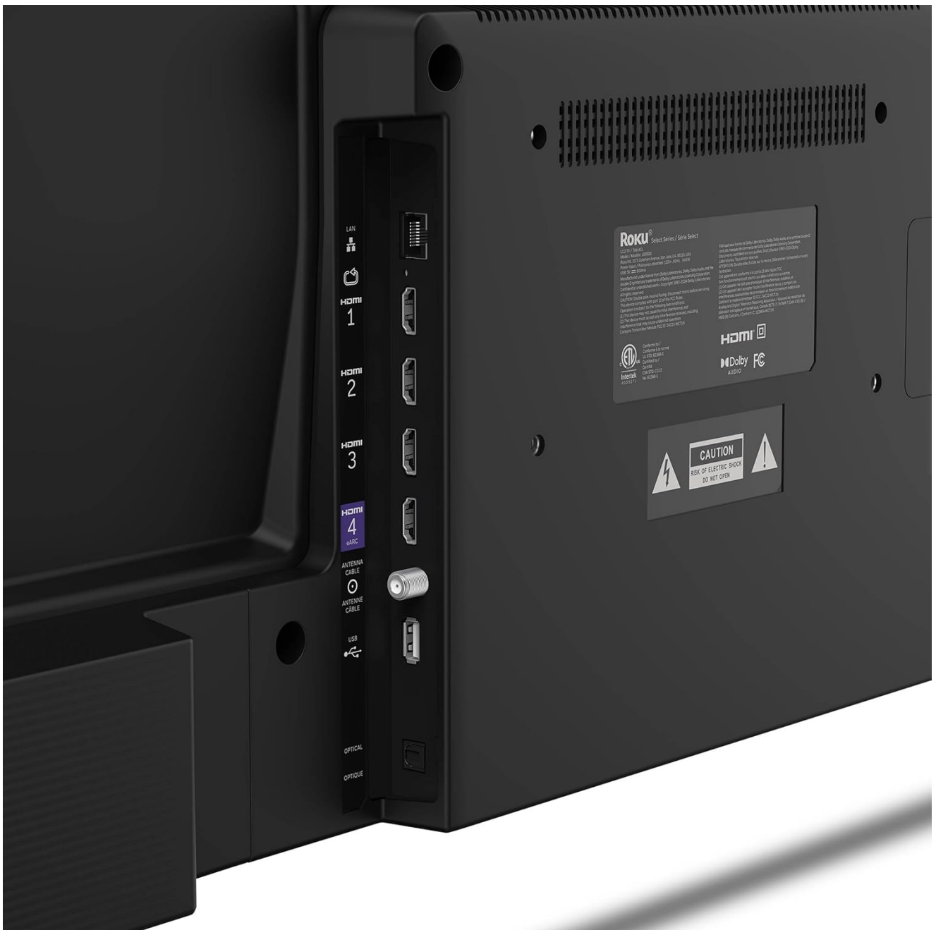
Figure 3: Rear panel connections including HDMI, USB, and network ports.
