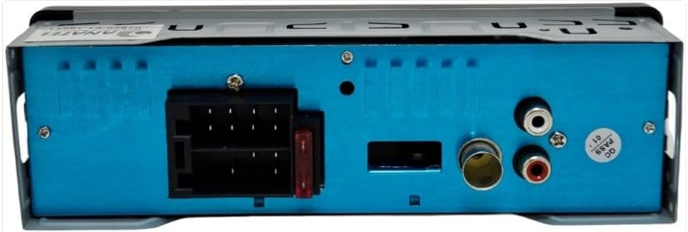
Image: Rear view of the H-TECH HT-1015 car radio, showing the main 16-pin wiring harness connector, antenna input, and two RCA audio output jacks (red and white).
