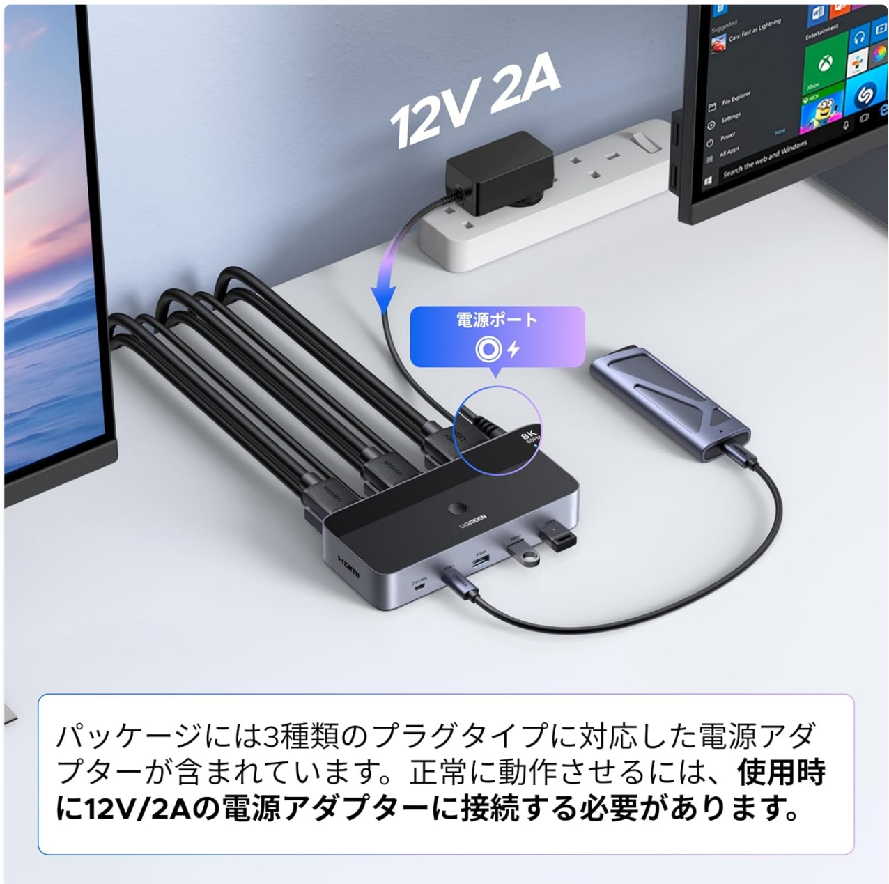
Image: Connecting the power adapter to the KVM switch.
