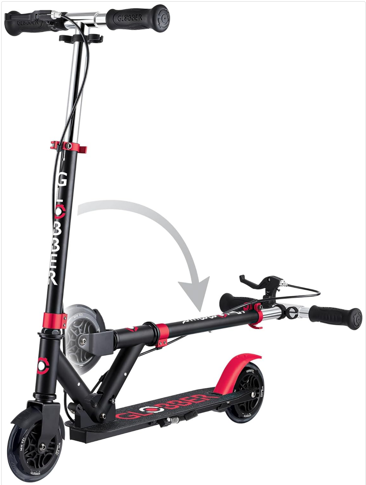
Figure 4.2: The scooter's folding mechanism in action.
