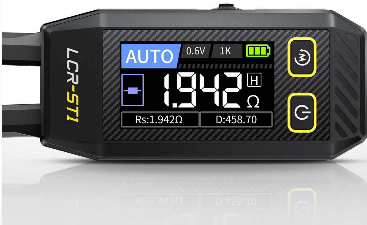
Image: A close-up of the FNIRSI LCR-ST1 Smart Tweezer display, showing a precision resistance measurement of 1.942 Ω and a dissipation factor (D) of 458.70.
