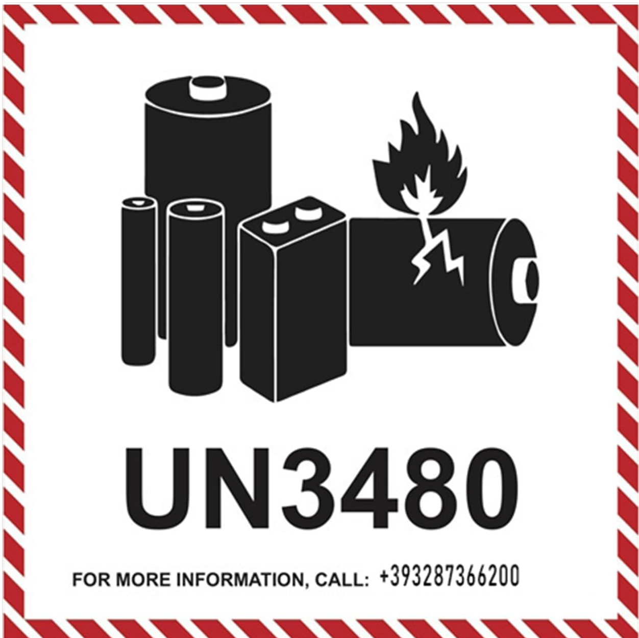
Image 3: UN3480 label indicating proper disposal and handling of lithium batteries.
