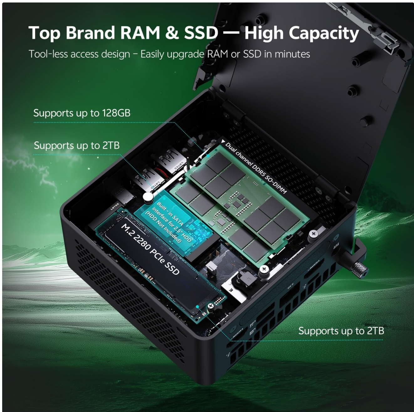
Figure 6.1.1: Internal layout of the ASUS NUC 15 Pro, illustrating the dual-channel DDR5 SO-DIMM slots for RAM and the M.2 2280 PCIe SSD slot, both designed for tool-less access and upgrades.
