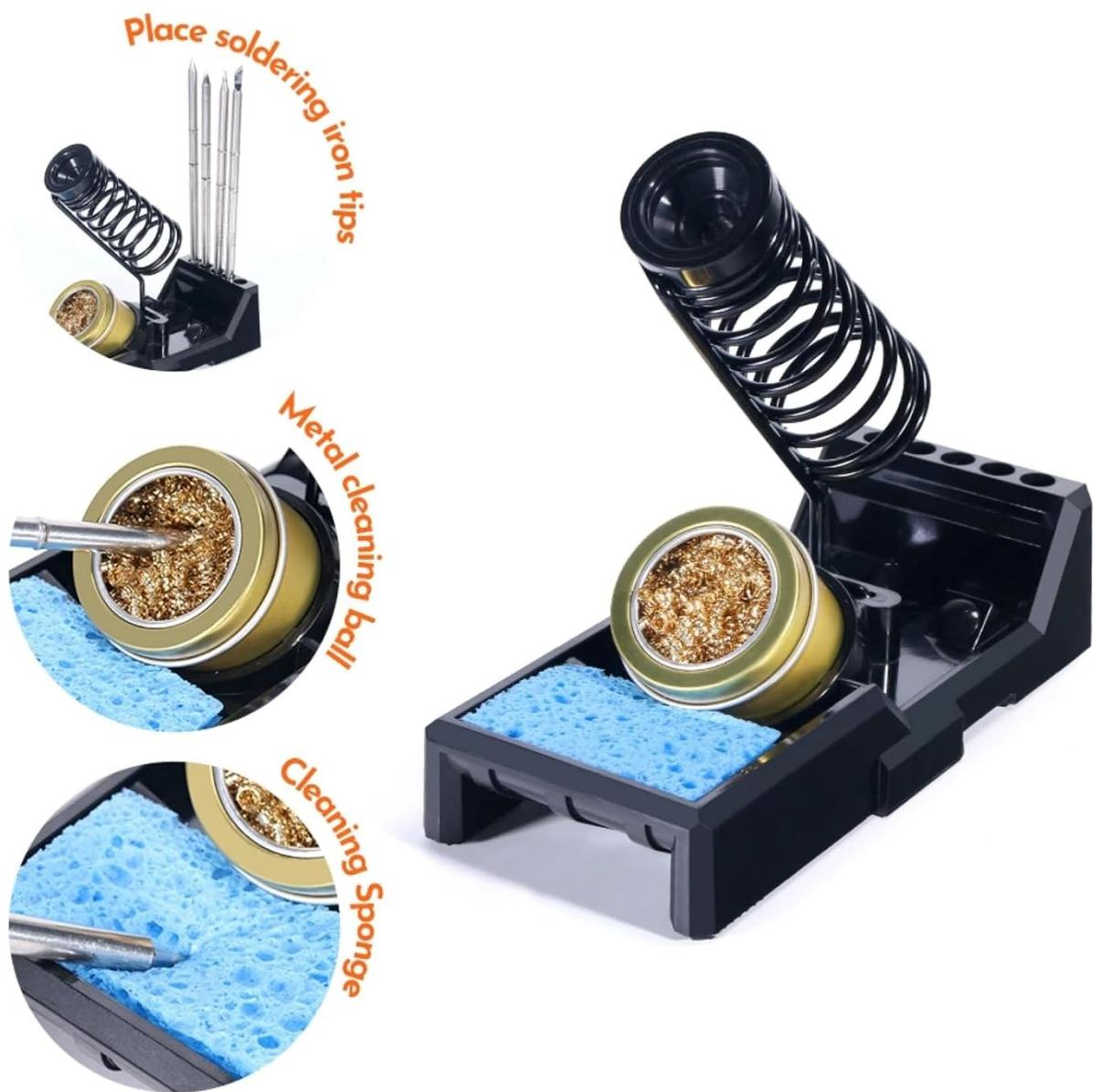
**Soldering Iron Stand and Cleaning Accessories:** The stand provides a safe place for the soldering iron and includes compartments for storing various soldering iron tips. It also features a metal cleaning ball for dry tip cleaning and a cleaning sponge for wet cleaning, both essential for maintaining tip longevity and performance.
