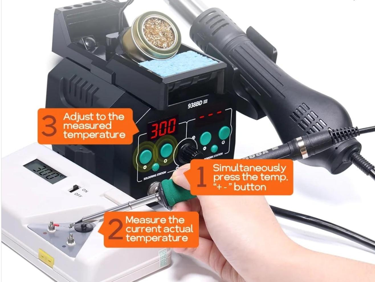
**Digital Temperature Calibration:** This image demonstrates the process of calibrating the temperature. First, simultaneously press the '+' and '-' buttons (1). Then, measure the current actual temperature using an external thermometer (2). Finally, adjust the displayed temperature to match the measured temperature (3).
