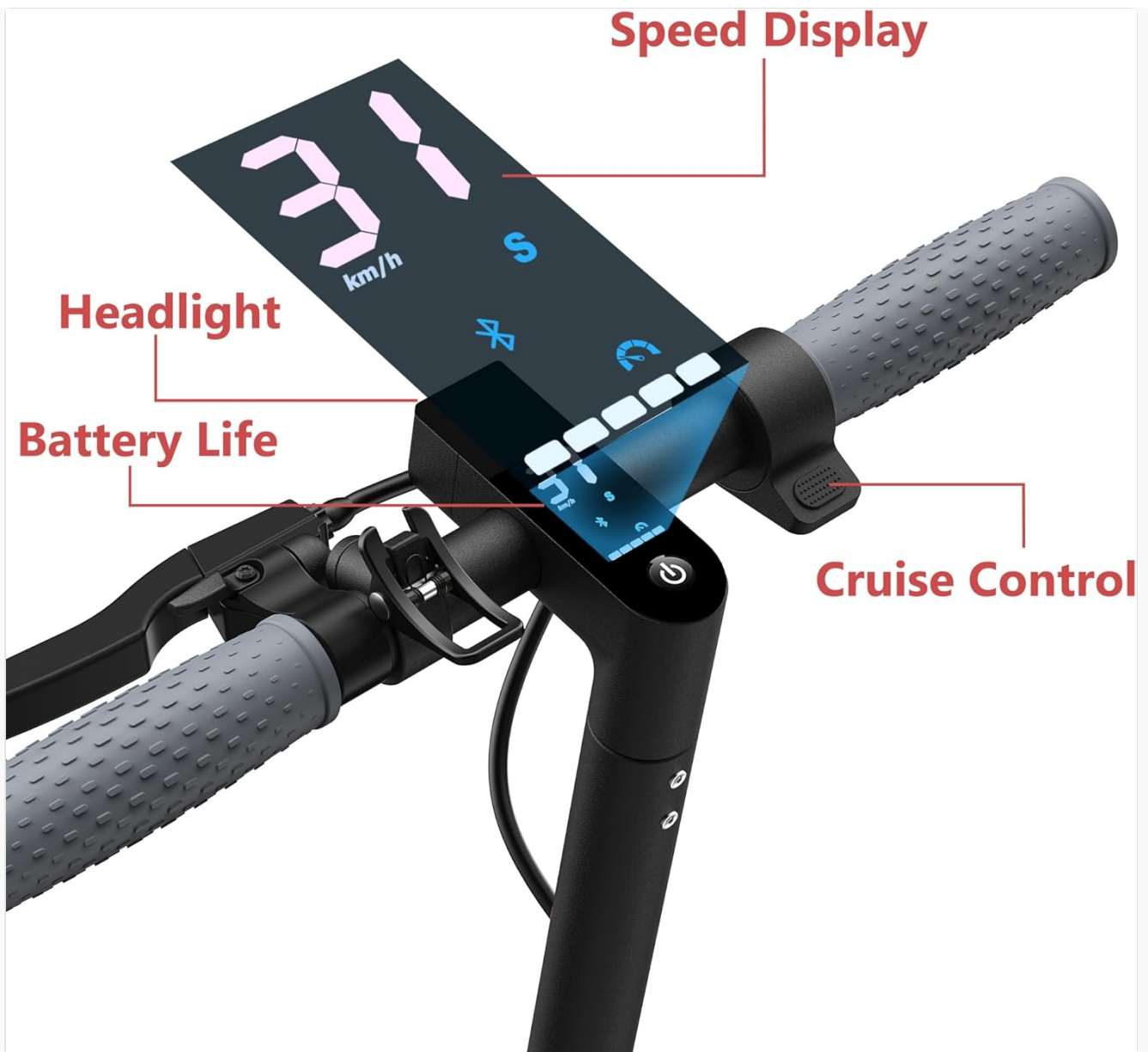
Image: A detailed view of the scooter's handlebar display, illustrating the speed readout, battery life indicator, headlight status, and cruise control function.
