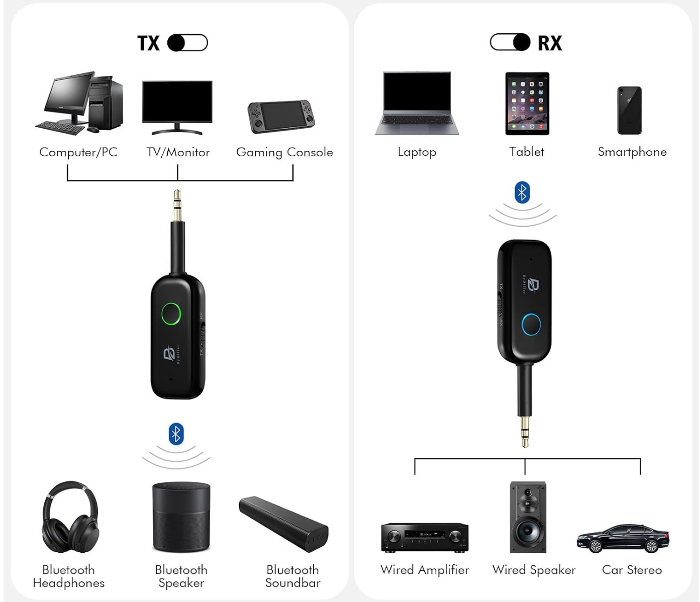
Image 2.2: Visual representation of the fnetic adapter in TX (Transmitter) mode, connecting to non-Bluetooth devices like TVs and PCs, and RX (Receiver) mode, connecting to wired audio systems like car stereos and speakers.
