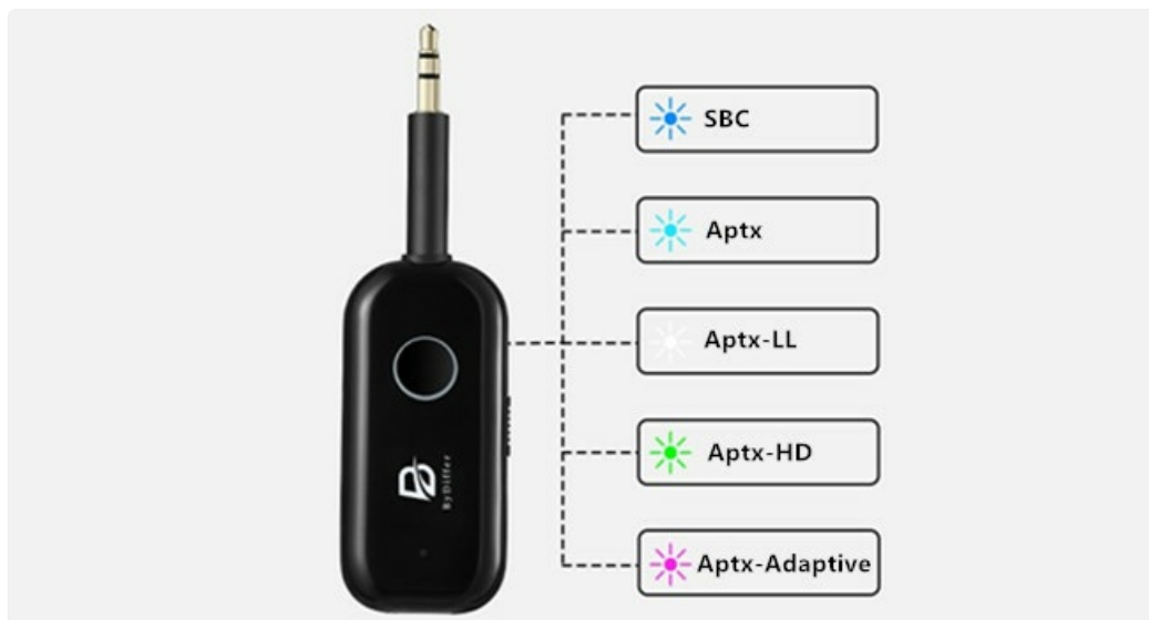
Image 3.9: Visual guide to the LED indicators for various audio codecs supported by the fnetic adapter, including SBC, aptX, aptX-LL, aptX-HD, and aptX-Adaptive.
