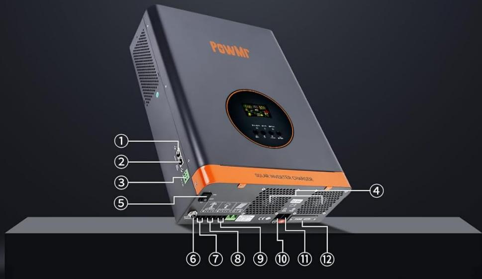
**Image:** PowMr 3000W Hybrid Solar Inverter showing various connection interfaces and protection functions. Key labels include RS232 communication interface, BMS/RS485 communication interface, Dry contact ports, Fan, Toggle switch, Input overcurrent protector, AC input, AC output, Photovoltaic input, Battery negative terminal, Battery positive terminal, and Battery circuit fuse.
