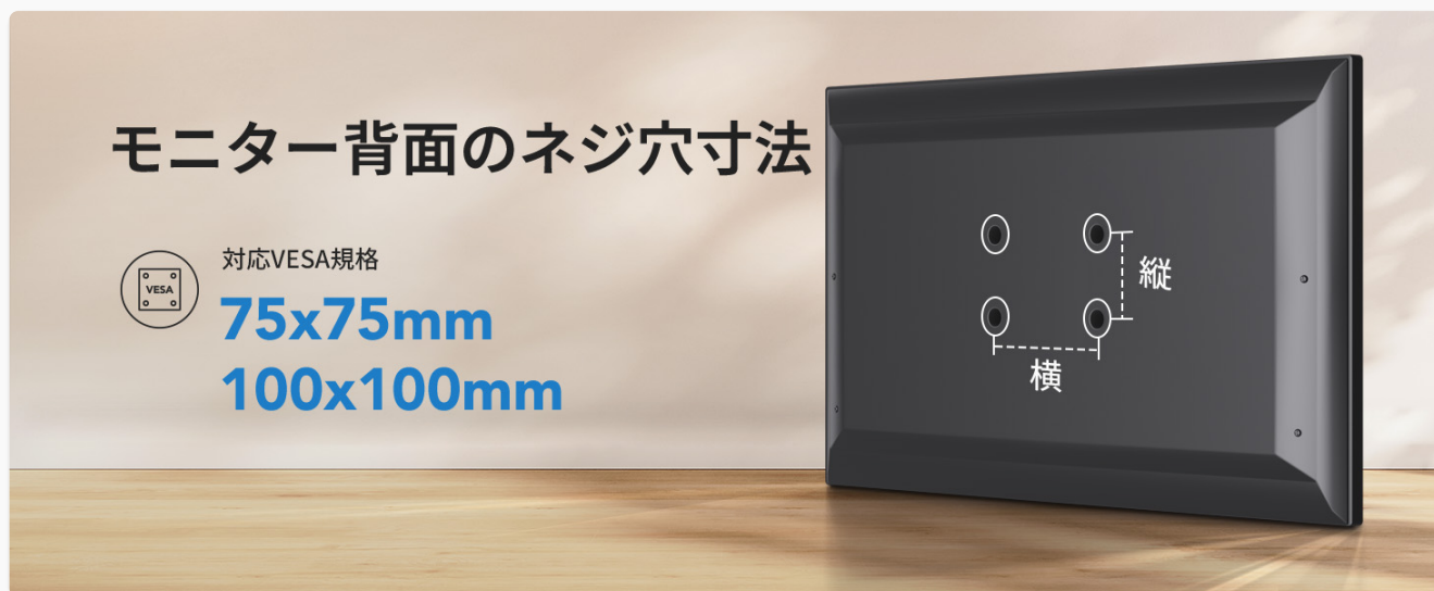
Image 5.2: VESA compatibility for monitor mounting.
