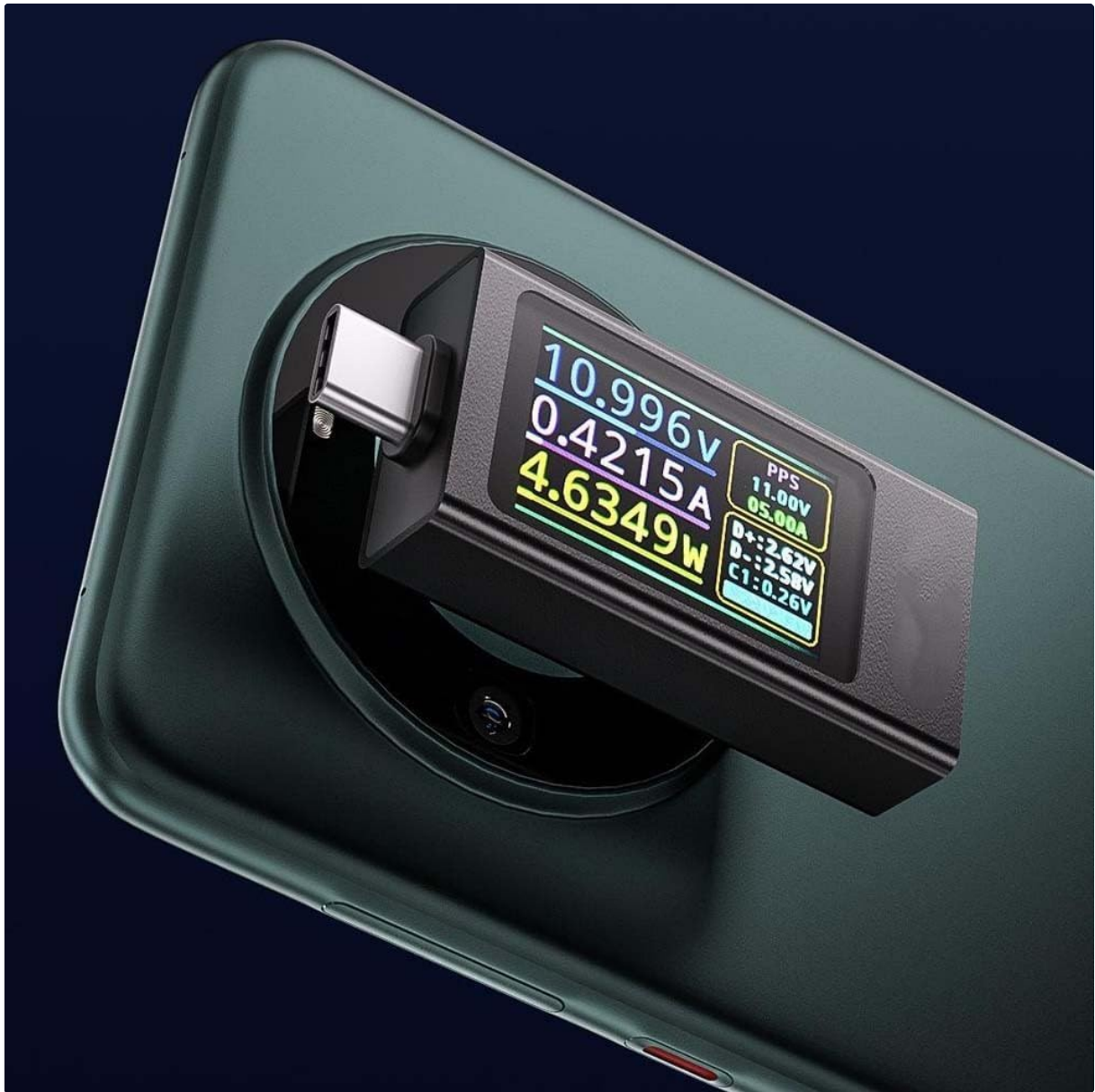
Figure 5.1: The KWS-X1 display showing real-time voltage, current, and power consumption, along with temperature. This is the primary monitoring screen for immediate feedback on charging status.
