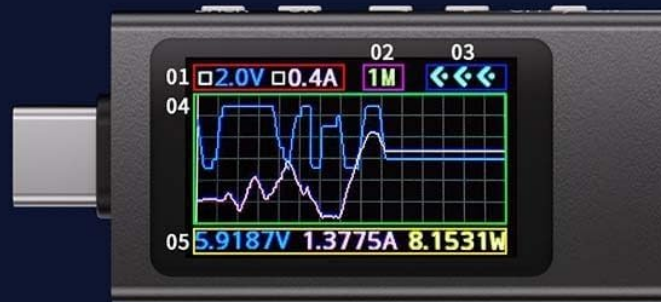
Figure 5.3: The KWS-X1 display showing advanced measurement modes, including a ripple measurement graph (top) indicating voltage stability over time, and a curve measurement graph (bottom) illustrating real-time voltage, current, and power fluctuations.
