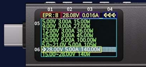
Figure 5.2: The KWS-X1 display showing the results of an automatic fast-charge protocol detection, listing supported protocols like PD 3.0, QC 3.0, and PD 3.1 with their respective voltage and wattage capabilities.
