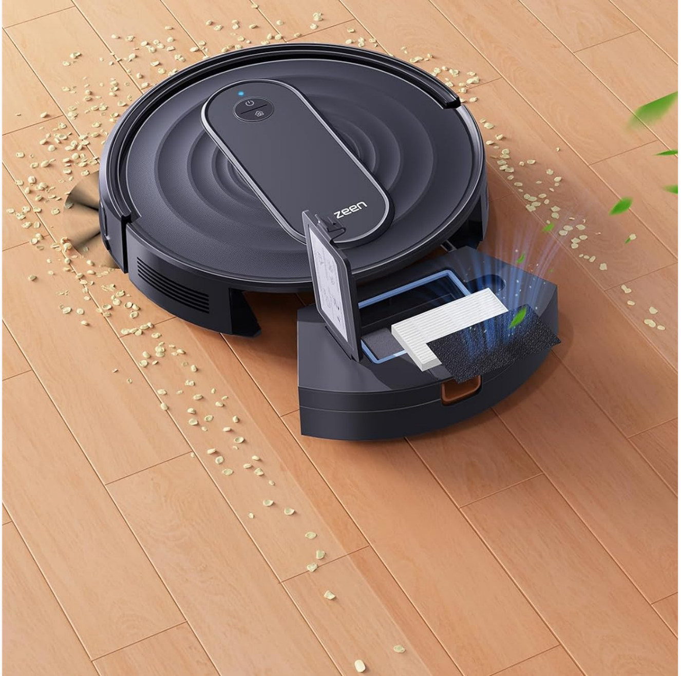
Figure 10: The R7's large dustbin and filter system.
