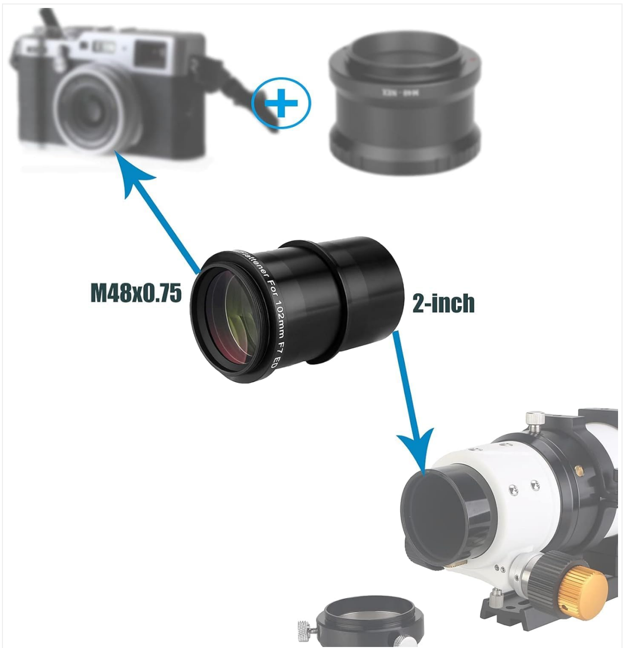
Image: Diagram showing the connection of the field flattener to a camera (M48x0.75 thread) and to the telescope's focuser (2-inch barrel).
