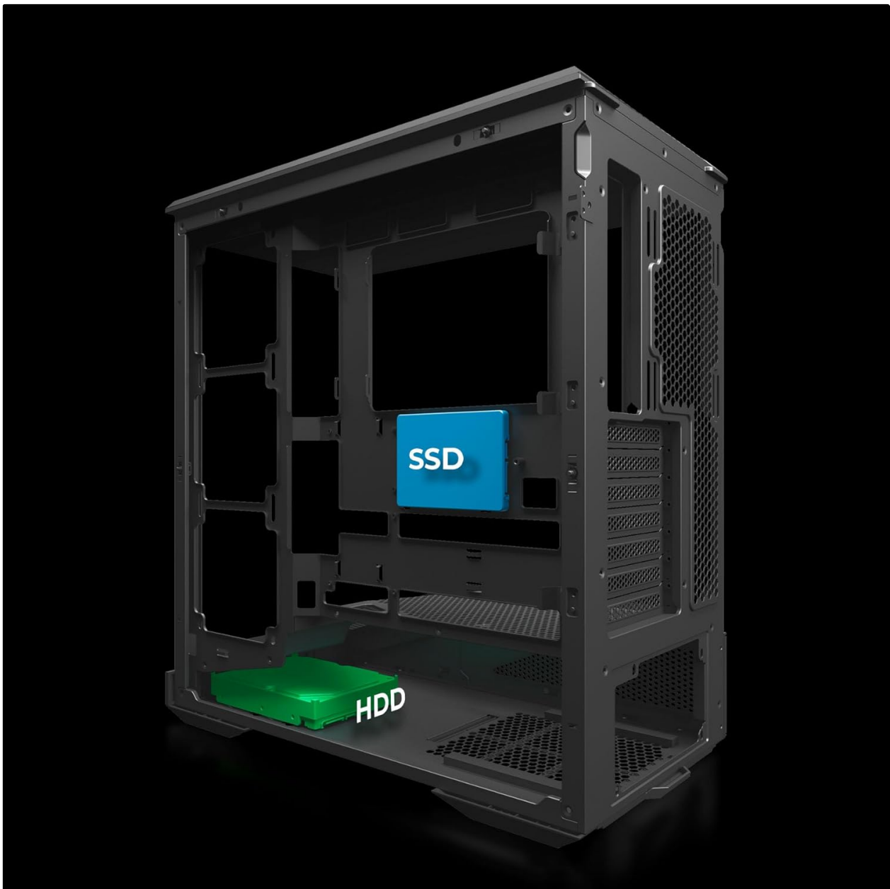
Image: Diagram illustrating the installation locations for SSD and HDD storage drives within the PC case.
