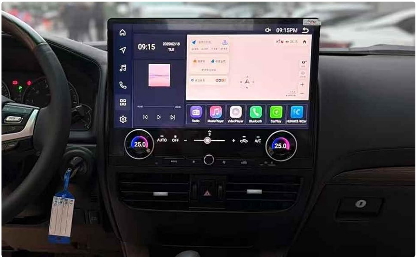
Figure 5.1: Main screen interface with climate control integration.
